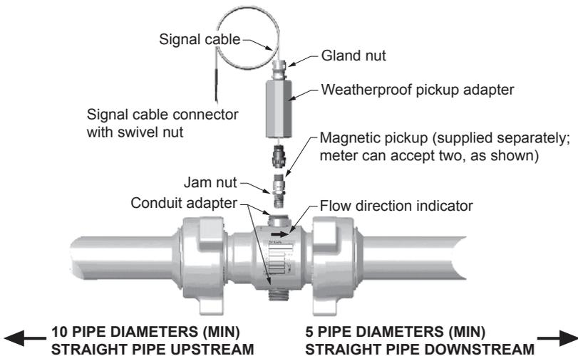
NOTE: Pipe must be of same nominal size as flowmeter end connection.
