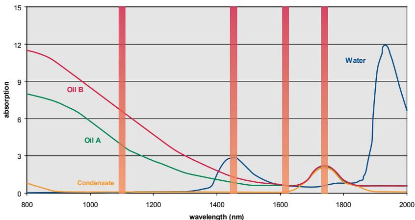
The graph shows several bands of infrared wavelengths that are absorbed by the components of the produced fluids.
